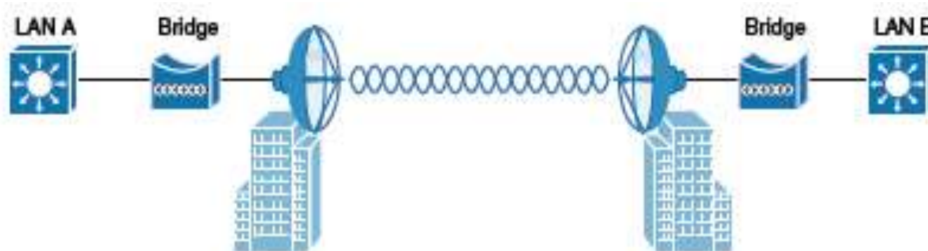
Figure 26-12 Point-to-Point Outdoor Bridge
