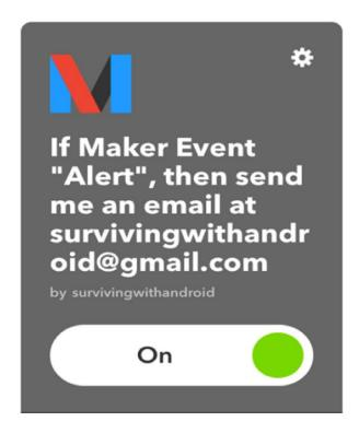
That's all. Now to trigger this event we have to call the URL as shown in the service configuration. The Arduino system will call this URL when the sensor detects an anomaly in the gas concentration.
