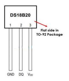
This sensor is frequently used in thermometers, thermostats, consumer electronics and industrial control systems.
