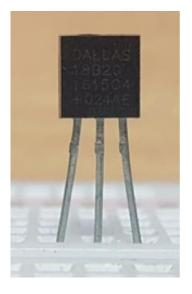
Coming to the sensor, DS18B20 is a Digital Thermometer which can measure temperatures in the range of -55  $^{\circ}$ C to +125  $^{\circ}$ C. The communication between the DS18B20 Sensor and the Microcontroller is through 1-Wire Communication (1-Wire Bus).
