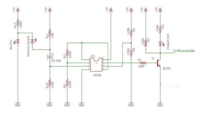
The above circuit shows the finger type heartbeat sensor, which works by detecting the pulses. Every heartbeat will alter the amount of blood in the finger and the light from the IR LED passing through the finger and thus detected by the Photo Diode will also vary.
