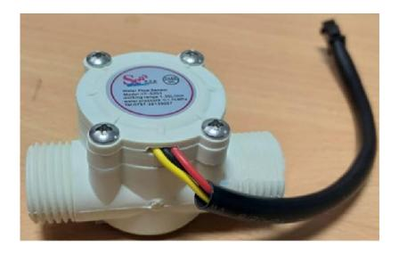
It has a plastic valve body with a rotor and a hall sensor circuit. It has three wires namely +5V (Red), GND (Black) and Output (Yellow). Since it works on +5V, it can be interfaced with any microcontroller like Arduino, for example.
