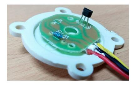
Based on the data sheet provided by Honeywell, the working of 460S Hall-effect sensor is as follows: when the South Pole of the magnet is towards the IC, then the output of the sensor is LOW and when the North Pole of the magnet is towards the IC, then the output is HIGH.
