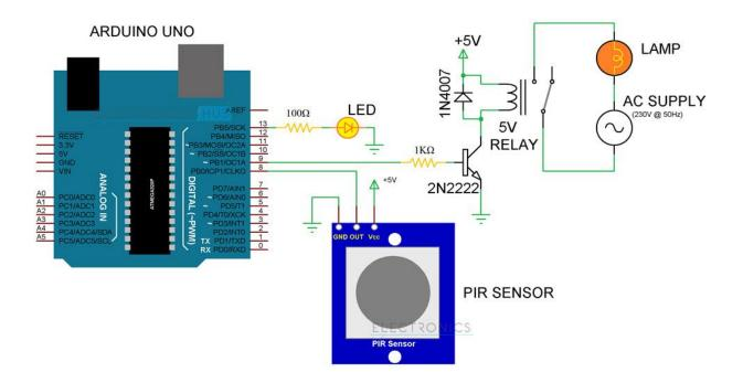
**CAUTION**: The project involves connection with 230V AC Mains (or 110V, depending on where you live!!!). Be extremely careful when connecting the bulb and Relay to mains supply. If you are unfamiliar with the connections, I strongly recommend having an adult supervision (or an expert supervision).
