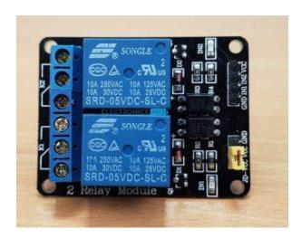
In order to control a single relay on the board, we need to use three pins of the relay module: VCC, GND and IN1.
